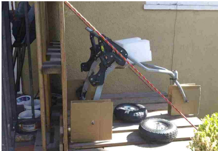
Figure 1: Mine, made from a discarded exercise stroller, mockup wheels mounted, 2 of 3 actual wheels also shown, unit seen partly assembled. Cost: ~$50.
